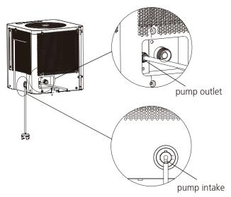
Note: The pump may be very noisy when it starts to work for 3~5 minutes. It is a normal sound.
